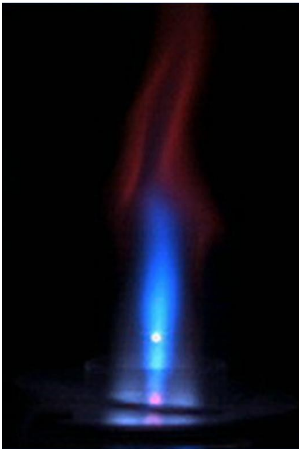
Figure 2b. Single high-speed image of the cloud surrounding a droplet produced from a Meinhard nebulizer at 1.9 mL/min. Notice the red YO emission in the core of the droplet and the neutral emission in the outer shell.
